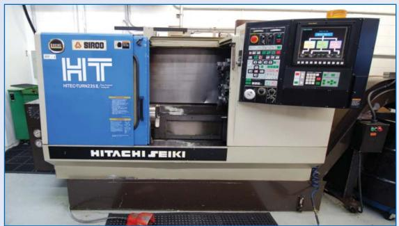
1994 HITACHI SEIKI HITEC TURN 23SII CNC Lathe With SEIKI MULTI CNC Control, 15.7" Swing, 24.8" Between Centers, 10" Chuck, 10 Station Turret, Tailstock, Tool Presetter, Chip Conveyor, 20 HP, 3,600 RPM, s/n HTS2644HL
