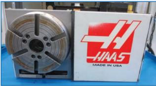
**HAAS** HRT-210, 4th axis rotary table with CNC Interfacing to M Functions, Variable Feedrates, RS232 Interface, Absolute or Incremental Programming, Auto Circle Division & Cabling
