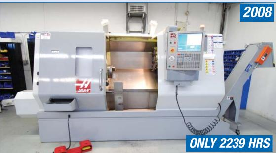
2008 HAAS SL-30T CNC Lathe HAAS CNC Control, 10" 3 Jaw Hydraulic & 10" 6 Jaw Chucks, 3,400 RPM Spindle, 3" Bore, 11.30" X-Axis, 36" Z-Axis, 12 Station Turret, 30 HP 2 Speed Drive, Tailstock, Tool Presetter, Parts Catcher, Chip Conveyor, 2 Worklights, 208/230 Volt, 3 Phase s/n 3084000 \*Only 2,239 Cutting Hrs.
