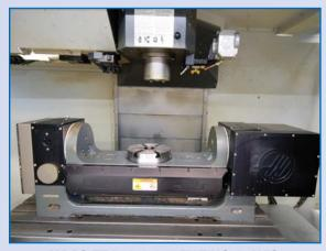
HAAS TR210 8.27" TILTING 2-AXIS TRUNNION ROTARY TABLE
