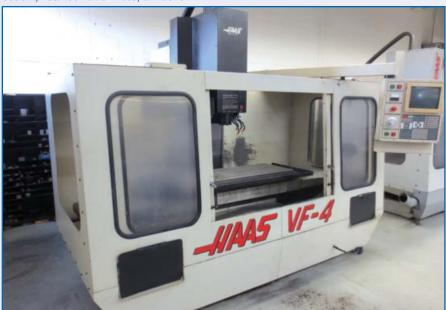
HAAS VF-4 CNC Vertical Machining Center With HAAS CNC Control, 18" X 52" Table, Travels: X-50" X, Y-20", Z-25", Cat 40, 4th Axis Ready, 20 ATC, 208/230 Volt, 3 Phase, S/N 2418
