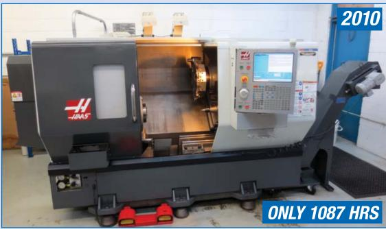
2010 HAAS ST20 CNC lathe With HAAS CNC Control, 8" 3 Jaw & 6" 3 Jaw Chucks,15" Swing X 23" Between Centers, 2" Bore, 4,000 RPM Spindle, 20 HP, 12 Station Turret, Tool Presetter, Parts Catcher, 2 Worklights, Coolant, Chip Conveyor, 195/260 Volt, 3 Phase, s/n 3085784 \*Only 1,087 Cutting Hrs.
