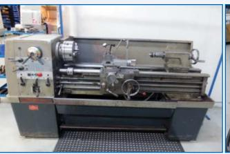
COLCHESTER Triumph 2000 - 600 Engine Lathe, With 18" Swing X 40" Between Centers, 2,000 Rpm, 3-Jaw Chuck, 2" Spindle Bore
