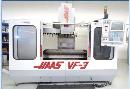
HAAS VF-3 CNC Vertical Machining Center, With HAAS CNC Control, 18" X 48" Table, Travels: X-40", Y-20", Z-25", Cat 40, 4th Axis Ready, 7,500 RPM, 24 ATC, 15 HP High Torque, Programmable Coolant, 208/230 Volt 3 Phase, S/N 5325
